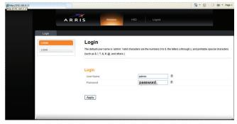
Connect your computer directly to the modem with an ethernet cable. If no ethernet connection is available, you may connect wirelessly as long as you are connected to the network you are changing. Open a browser and enter **192.168.0.1** in the address bar and press enter. The username is "admin" and the password is "password". Enter that and click "apply".
